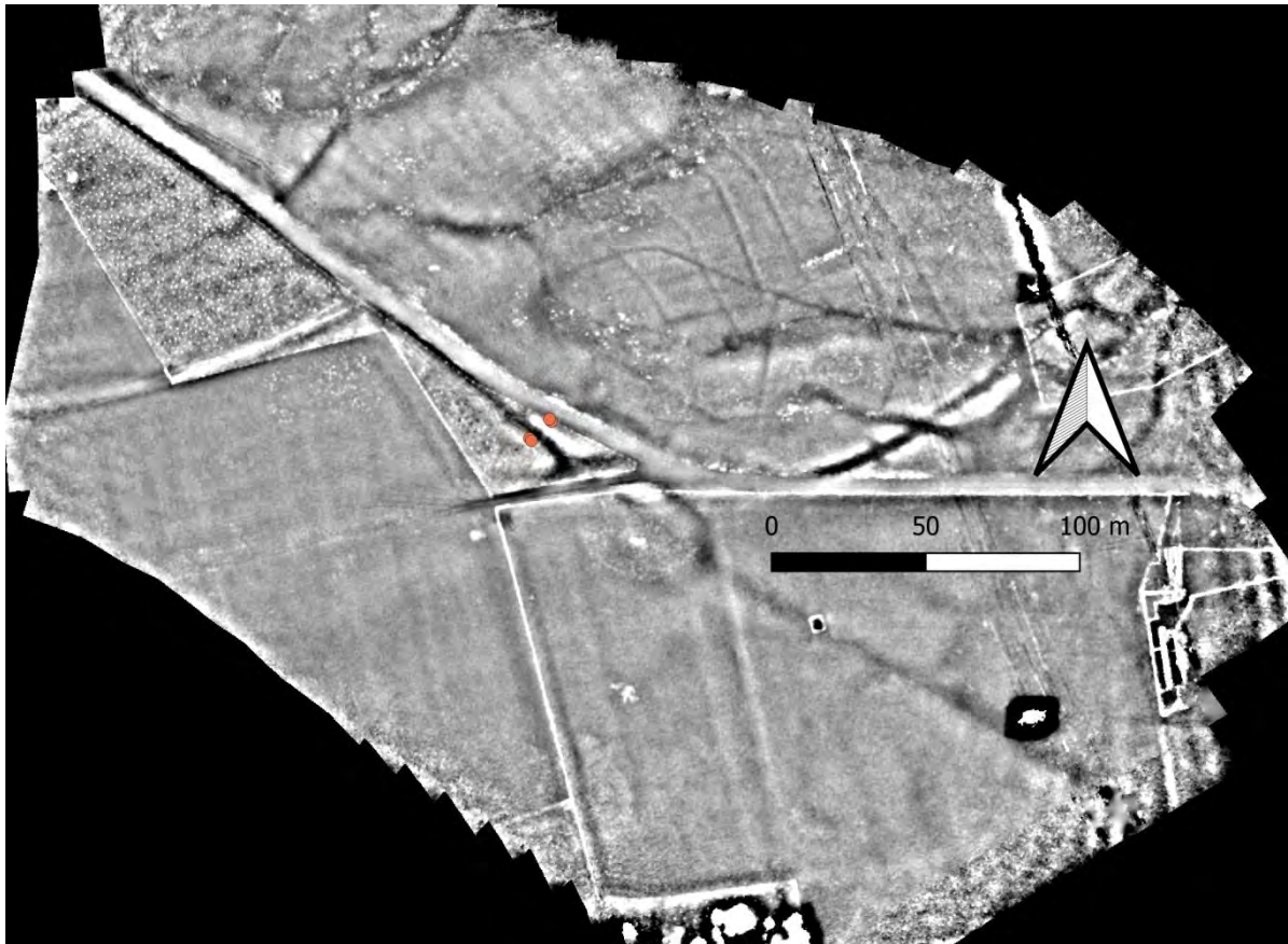
Figure 9 LRM of the earthwork with Trench 1 marked by red spots on the image. The earthwork is revealed in high relief with this view showing the ditch in black and the bank in white. The earthwork's ditch continues in the arable field as a dark line to the southeast edge of the image, showing the benefit of using the local relief model in picking up slight changes in the ground surface. The breadth of the bank of the earthwork at the top left has been exaggerated by the addition of road metalling to make a farm track which makes use of hard base provided by the bank. The track metalling also runs across and obscures part of the secondary earthwork that runs in an arc to the northeast. The earthwork that abuts the excavated earthwork on its west is highlighted as a vivid, slightly curving white line.
